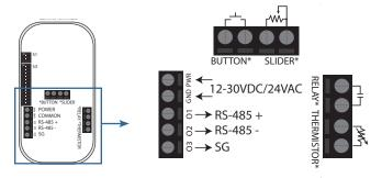
NOTE: A 120  $\Omega$  termination resistance may be added in parallel with the RS-485 +/- by moving the very top DIP switch (DIP 1) to the left position. See "DIP Configuration" section for more information.
